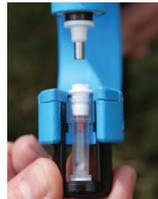
**2a.** Remove the TSU tube from the pliers by opening the retention ring and sliding out the tube.
