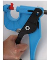
**3b.** You now have completely grabbed the needle. After the needle is inserted into the piston you can release the handles.
