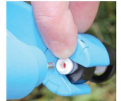
In the used TSU a clear RED plunger will be visible indicating the tube already contains a sample and can't be used again.
