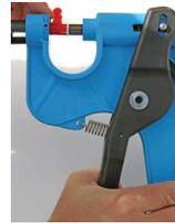
**3a.** Carefully squeeze the plier handles until the large piston comes to a stop against the red connection piece.
