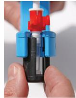
**2d.** After insertion of the TSU close the retention ring to lock the tube.
