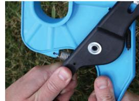
**3.** Remove the used needle from the pliers by pulling the handles apart. This will loosen the needle and make it easy to remove. The needle is no longer of use as it no longer contains the red plunger.
