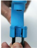
**2a.** Open the TSU retention ring on the pliers.
